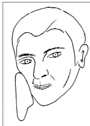
FIG. 1 Sketch portraying the contact angle between face and cheek piece which causes the left eye to be higher than the right when using offset sights. "Cast off" in the stock causes the right eye to seem to be too far left to line up with the action-barrel axis in this diagram.
