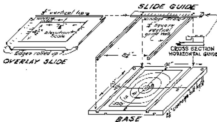
*Fig. 5 Schematic diagram of the components in one version of the Plotamatic. In other versions the essential horizontal and vertical movements of the overlay are provided by different mechanisms.*
